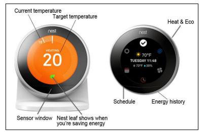
If the heating is already on, you can turn the temperature up or down by turning the outer ring: clockwise for hotter, anticlockwise for lower heat.
